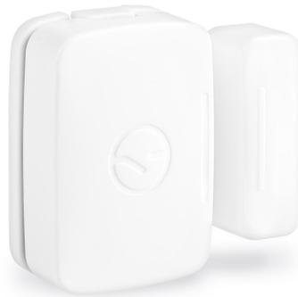
Figura 3.8: Sensor *Smartsense Open/Closed*
