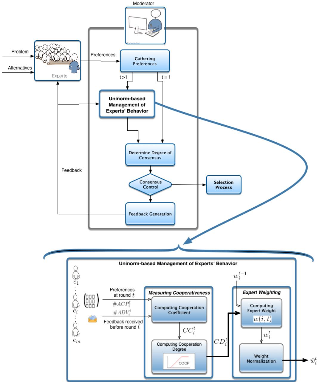
**Figure A.3:** Scheme of the uninorm-based method for managing experts' behaviours in large scale consensus reaching processes.
