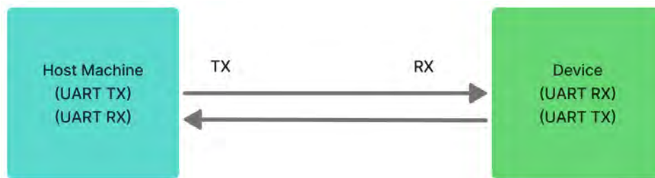
Figure 2.14: UART Communication. Source: Own creation
